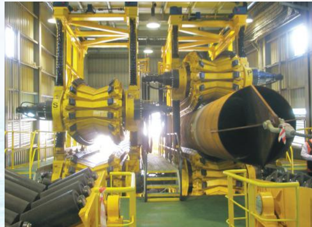
2 x 80 ton Hydraulic Driven Pipe Tensioner
